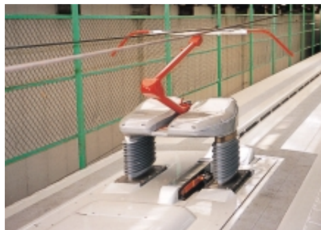
A new single-arm pantograph and insulator
