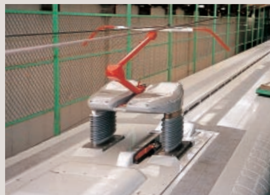
Single-arm pantograph and insulator designed to minimize noise
