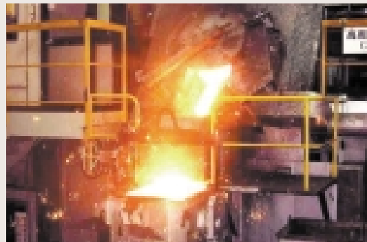
In the Nagano Rolling Stock workshop, waste metal is recycled into parts for railcar brakes and others.
