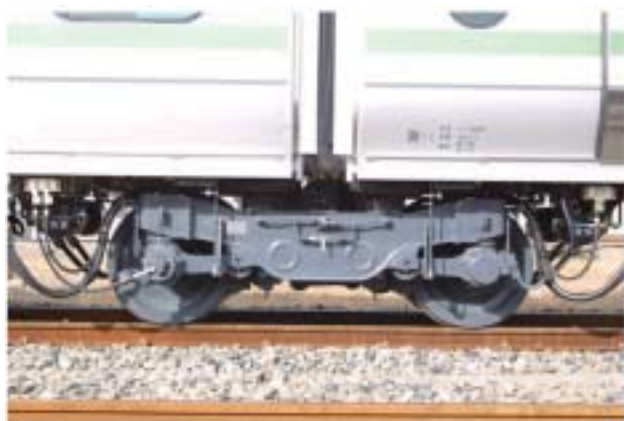
Fig.4: External Appearance of the Articulated Part
