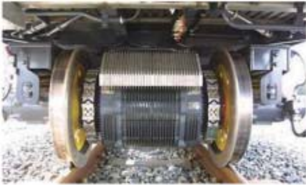
Fig.7: External Appearance of the Propulsion Direct Drive Motor (DDM)
