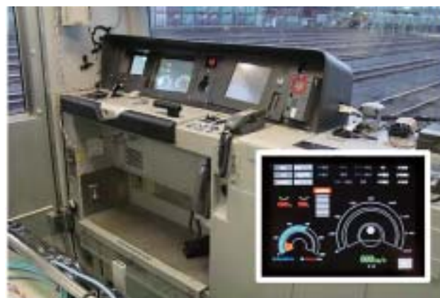
Fig.11: Monitoring Equipment in the Motorman's Cab utilizing AIMS (Advanced Train Information Management System)
