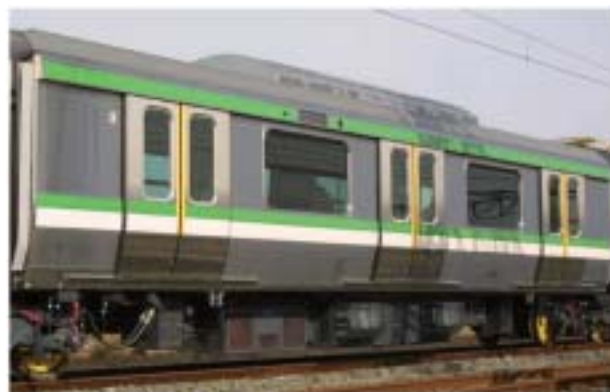
Fig.6: Double Skin Train Body using Stainless Steel
