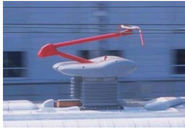
Fig.37: Hayate Low Noise Pantograph
