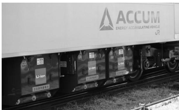
Fig. 4 Traction Circuit Storage Battery Box
