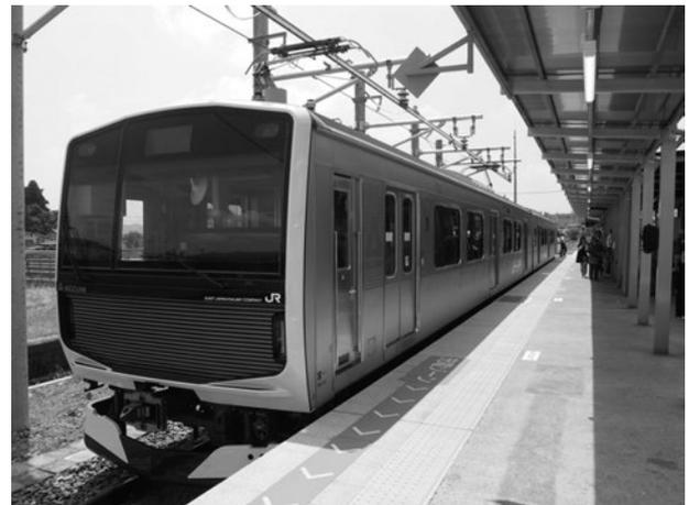
Fig. 13 Series EV-E301 Charging Batteries at Karasuyama Station
