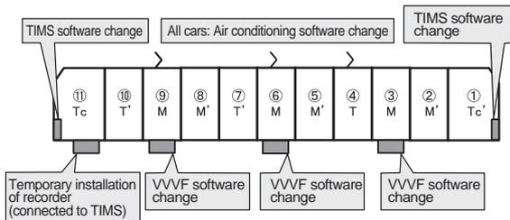
Fig. 1 Measurement System Configuration on the Yamanote Line
