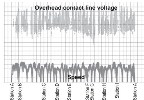
Fig. 3 Overhead Contact Line Voltage Fluctuation (at regeneration)
