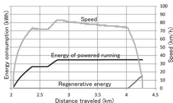
(b) Min. electric energy consumed for running (20.2 kWh)
