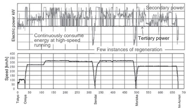
Fig. 4 Comparison of Energy Consumption in Constant Speed Control
