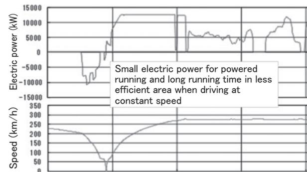
Fig. 10 Electric Power Generation at Constant Speed Driving
