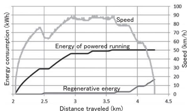
(a) Max. electric energy consumed for running (33.7 kWh)
