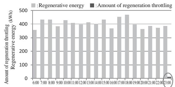
Fig. 2 Regeneration Throttling per Hour
