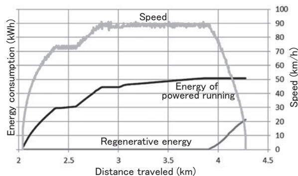
(b) Min. electric energy consumed for running (18.3 kWh)
