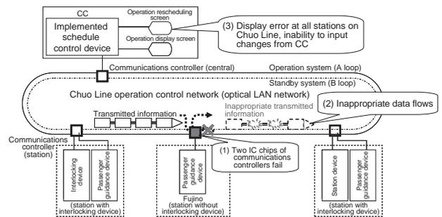
Fig. 4 ATOS Network Communications Disruption at Fujino Station on the Chuo Line
