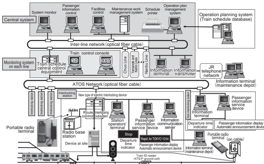
Fig. 1 Overview of the Autonomous Decentralized Transport Operation Control System (ATOS)
