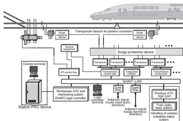
Fig. 3 Overview of Digital ATC System (DS-ATC)
