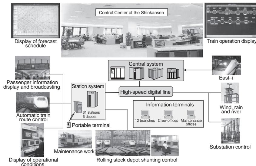
Fig. 2 Overview of Computerized Safety, Maintenance and Operation Systems of Shinkansen (COMTRAC)
