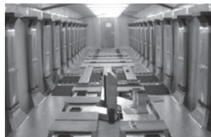
Fig. 1 Air Conditioning Ducts in Car Body Mockup Model
