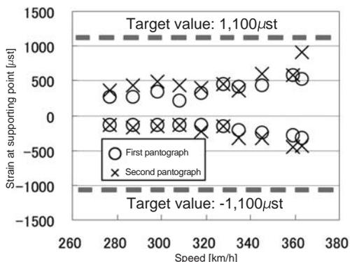
Fig. 8 Strain in Contact Wire (in coupled operation test, with improved line system ③)
