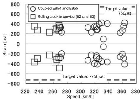
Fig. 11 Measurement Results of Snow Melting Device at Turnout
