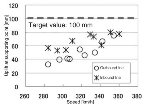
Fig. 2 Uplift of Contact Wire (in passing test, with improved line system ③)
