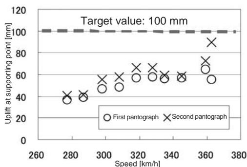
Fig. 7 Uplift of Contact Wire (in coupled operation test, with improved line system ③)
