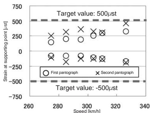
Fig. 6 Strain in Contact Wire (in coupled operation test, with higher tension line system ②)
