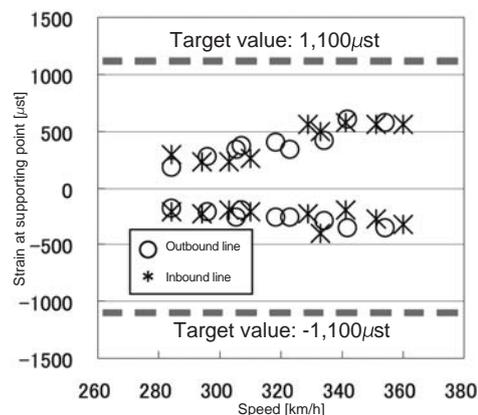
Fig. 3 Strain in Contact Wire (in passing test, with improved line system ③)
