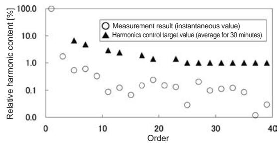
Fig. 12 Measurement Results for Relative Harmonic Content (Type E954, powered running current: 486A)
