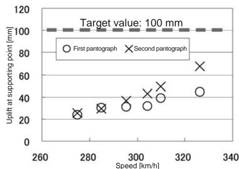
Fig. 5 Uplift of Contact Wire (in the coupled operation test, with higher tension line system ②)
