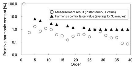
Fig. 13 Measurement Results for Relative Harmonic Content (Type E954, regenerative current: 486A)
