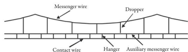
Fig. 1 Structure of Heavy Compound Catenary
