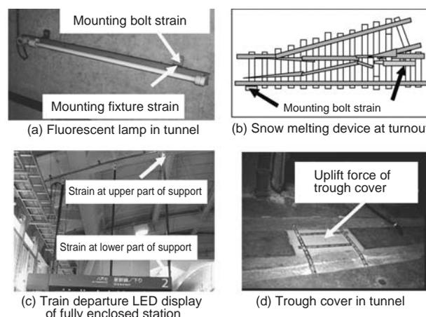
Fig. 9 Measured Lighting and Power Equipment
