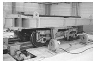
Fig. 6 Bogie Bench Testing
