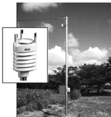
Fig. 11 High-Density Ground-Level Weather Observer (Able to Measure Direction and Speed of Wind, Temperature, Air Pressure, Precipitation and Humidity)
