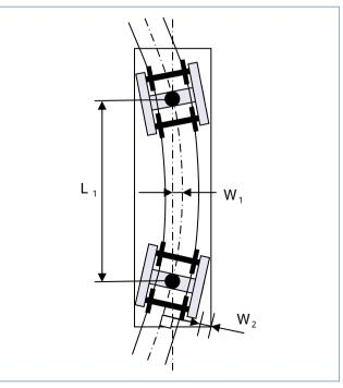
Fig. 8 Deviation on the curve
