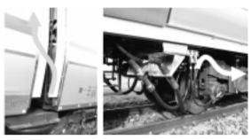
Fig. 12 End-to-end cable routing (left) and bogie-internal cable routing (right)
