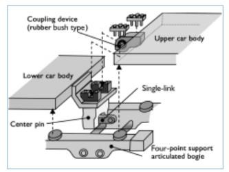
Fig. 7 Installation of four-point support articulated bogie
