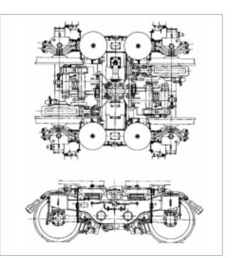
Fig. 6 Four-point support articulated bogie
