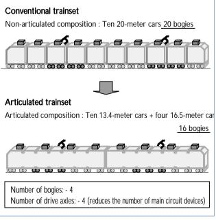
Fig. 1 Reduced number of bogies in articulated structure
