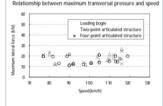
Fig. 13 Derailment coefficient and maximum lateral force (R = 800 m and C = 95 mm)
