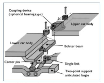
Fig. 5 Mounting the two-point support articulated bogie
