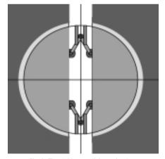
Fig. 9 Turntable type link mechanism
