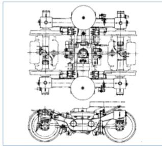
Fig. 3 Two-point support articulated bogie
