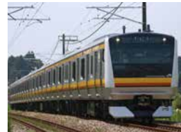
E233 series: VVVF inverter cars for commuter and suburban transportation
