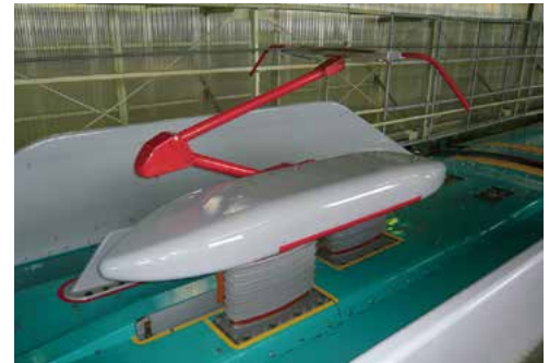
E5 Series trains have low-noise pantographs
