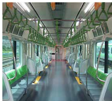
LED railcar lighting
