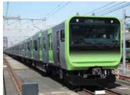
E235 series: New rolling stock models equipped with state-of-the-art train information management system were introduced on the Yamanote Line
