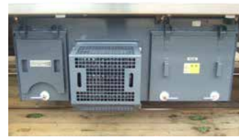
Main controller (VVVF inverter system)
