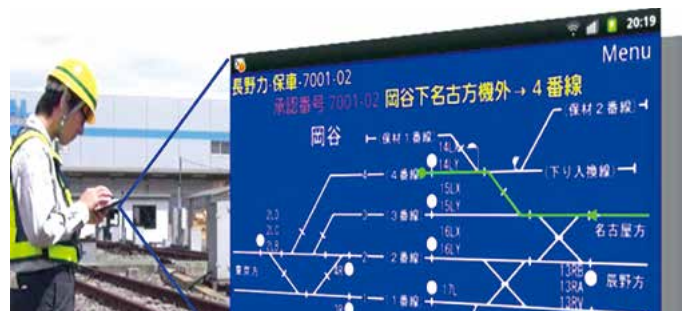
Visualization of maintenance work procedures
