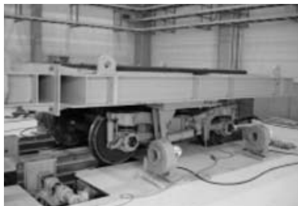
Fig.10: Long term endurance test (bogie testing device)
