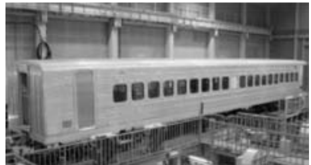
Fig.9: Test on rolling stock test rig (Railway Technical Research Institute)
